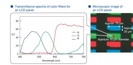
A circular 10  $\mu m$  aperture was applied for each subpixel of red, green and blue (R, G, B).
