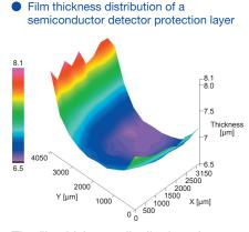
The film thickness distribution of a semiconductor detector protection layer was calculated from the interference wave shape in the NIR region.
