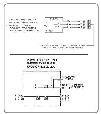
Transmitter Wiring Diagram
