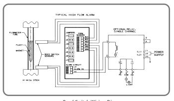
Reed Switch Wiring Diagram
