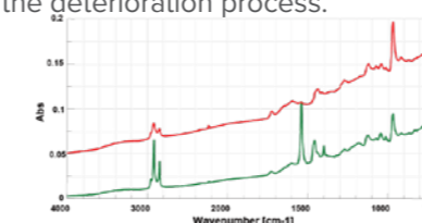
Spectrum of rubbers (Green: Normal rubber, Red: Deteriorated rubber)
